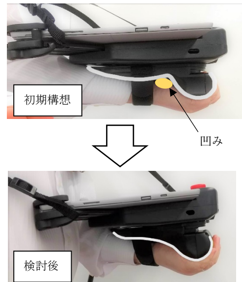
図8 検討前後のグリップ形状 Fig.8 Grip shape before and after consideration
