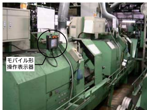
図5 単能旋盤機への導入例 Fig.5 An introduction example to Simple lathe machine.
