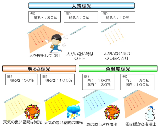
図7 調光制御の概略 Fig.7 Dimming control outline
