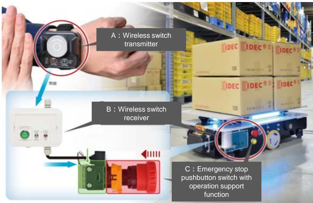
“Emergency-stop assist system” consisting of three devices, A, B, and C.
