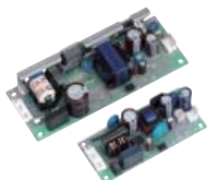
Constant current power supplies like these are optimal for LED illumination needs
